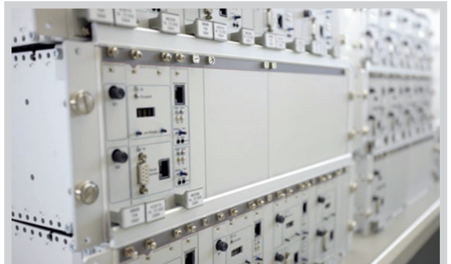
Figure 6: ACS2000 – centralised architecture with fail-safe relay interface
